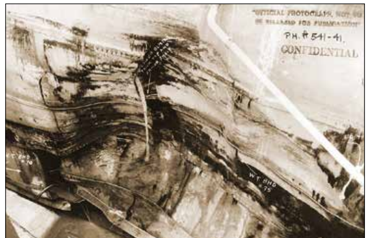
Damage to the USS Arizona after colliding with USS Oklahoma. The ship entered drydock for repairs, which postponed a trip to Washington and remained at Pearl Harbor until December 7, 1941.
