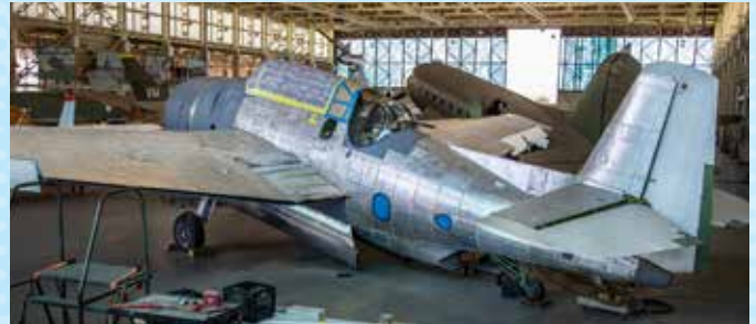
TBM Avenger currently under restoration.
